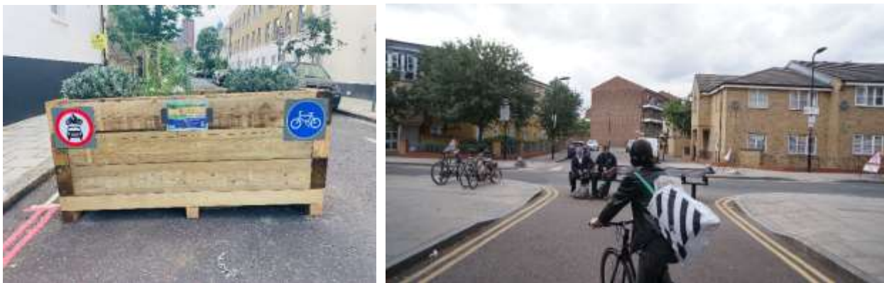
Figure 6-7: Examples of ‘modal filters’ used to remove vehicle access and enforce ‘Low Traffic Neighbourhoods’ (LTNs) (Richborne Terrace using community adopted planters (left) and xxx using a bench instead of bollards (right))
